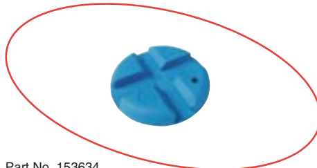
Part No. 153634 Cable support tool: While mounting the connector this unique rubber tool gives you a good grip of the cable, and with no risk of damaging the cable. Support cables with dimensions 3-12 mm
