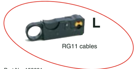
Part No. 153602 Stripping tools: With rotary cable strippers, preparation of cable is reduced to a single operation resulting in precise stripping in the dimensions matching exactly with the connector. The non-expensive stripping tools are pre-adjusted for RG6 and RG11 cables respectively.
