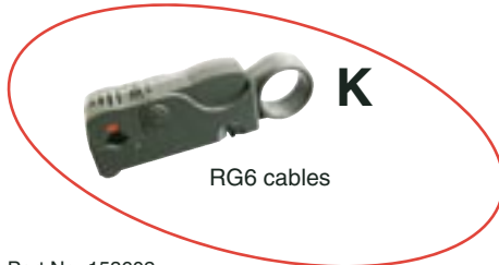
Part No. 153602 Stripping tools: With rotary cable strippers, preparation of cable is reduced to a single operation resulting in precise stripping in the dimensions matching exactly with the connector. The non-expensive stripping tools are pre-adjusted for RG6 and RG11 cables respectively.
