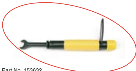
Part No. 153632 Torque wrench spanner: The spanner ensures a proper installation in accordance with SCTE standards, minimizing the risk of heavy screening leakage. When using F-connectors outdoors SCTE recommends a torque of 3,4 - 5,6 Nm.
